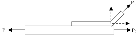
Fig. 17 Free body diagram of the attachment and adherend.
